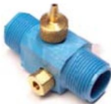
Air injection iron filters use oxygen in the air to oxidize iron in water. A small venturi type air injector is installed between the pump and pressure tank to draw the air into the water. The iron oxidizes to form rust particles, which are then strained out by a filter medium (birm).
